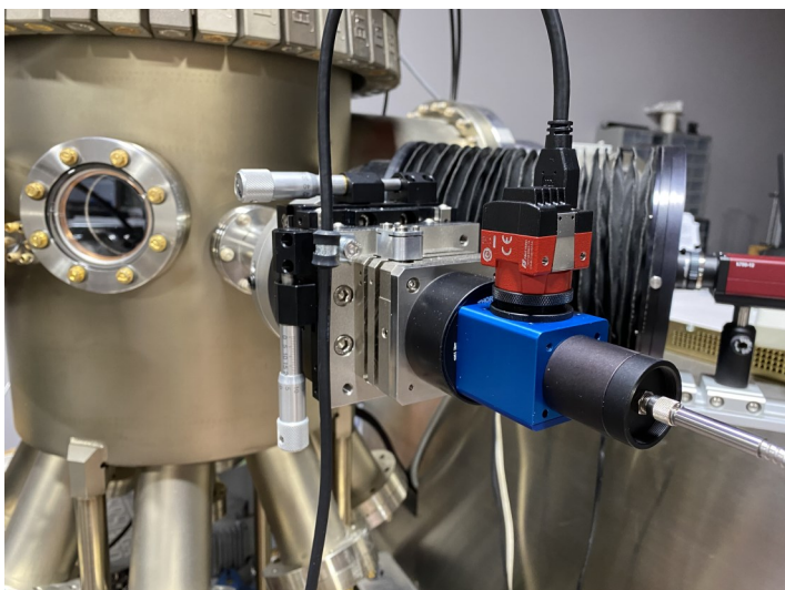
kSA ACE detector with beam monitoring camera for ease of alignment and real-time characterization of beam profile.
