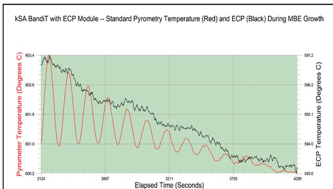
**Figure 2: a) Temperature trace for MBE growth of AlGaAs on a GaAs substrate, comparing kSA ECP data and classical pyrometer data.**
