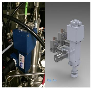
Figure 1: a) Temperature trace for GaN growth on Si comparing kSA ECP Module data (blue) and classical pyrometer data (red). b) Image of kSA ECP module integration with kSA ICE system and its installation on a D-180 MOCVD reactor.
