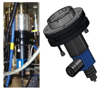
Figure 2: b) Image of the ECP module integration with kSA Bandit detector head, and its installation on a production MBE reactor.
