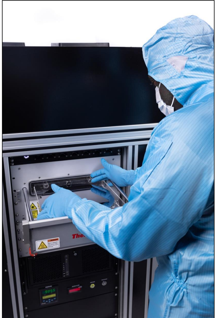
Sample loading of 300 mm wafer for a kSA MOS ThermalScan Model TS300-HT.
