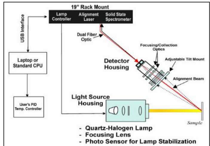
Figure 2: kSA BandiT Two-Port Reflection Mode Configuration.
