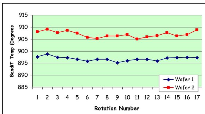
Figure 8: Wafer center point temperature extracted for two separate wafers on susceptor.
