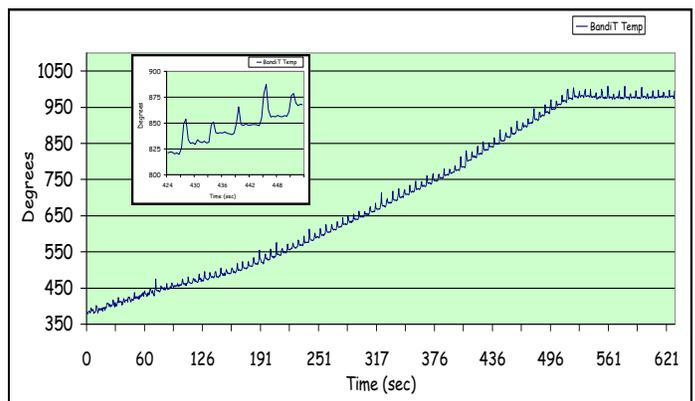
Figure 5: MOCVD temperature ramp and stabilization with multi wafer temperature detection.
