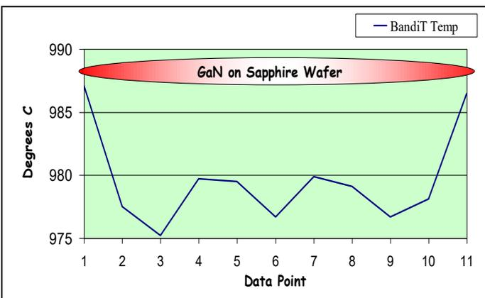
Figure 6: 3" Spatially resolved wafer surface temperature during MOCVD planetary rotation.
