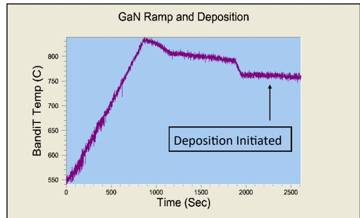
Figure 11 : GaN deposition with no change in temperature signal.
