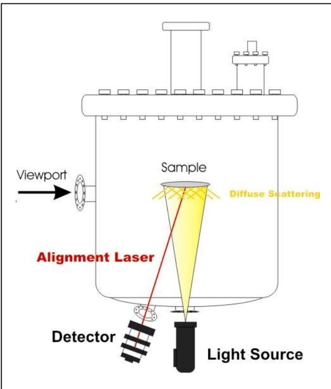
Figure 9 : BandiT mounted on Veeco GEN200 MBE.
