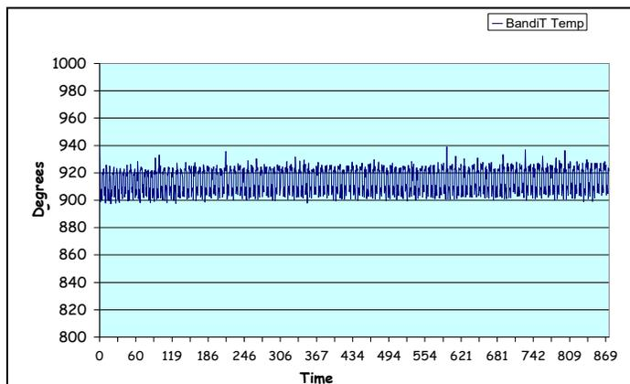
Figure 7: 1000 Å InGaN growth on single wafer GaN. Temperature gradients across wafer yield oscillations.
