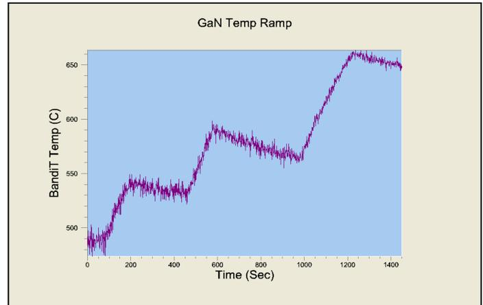
Figure 10: MBE GaN temperature measurement during 50 °C ramps.
